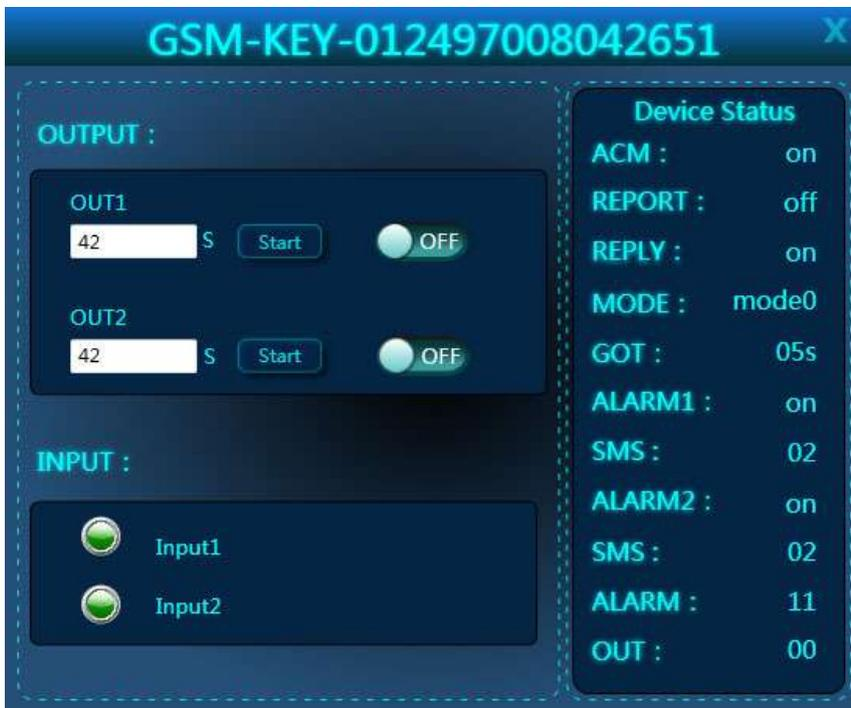
On the panel, you can remote control the relay output to ON or OFF with the ON or OFF switch for each relay output.
